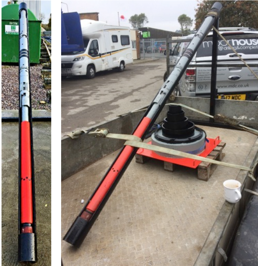
Completion model to scale: sliding sleeve (red) and production packer (grey). The model shows the actual 45° inclination of the HH-1 well within the KL3 and KL4.
